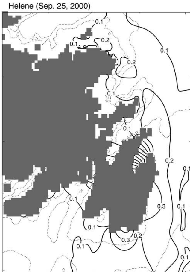
Figure 9. Maximum set-up in adjusted sea level near southeastern Newfoundland in the standard Tropical Storm Helene model run. The contour interval is 0.1 m.
